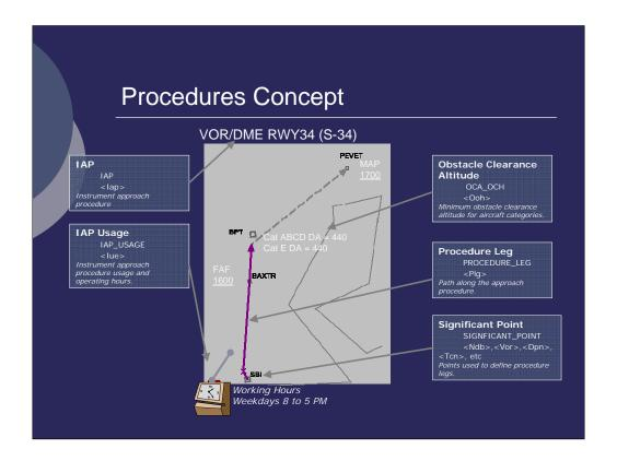
The Procedures data concept area defines instrument approach procedures, departure procedures and standard terminal arrive routes. AIXM uses the ARINC 424 standard as the basis for the data model used to create procedures in AICM and AIXM.
