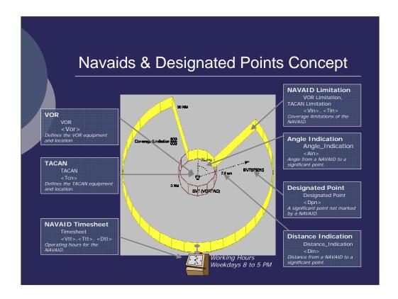
The NAVAID and Points Domain defines points in space used for navigational and air traffic control purposes. An abstract concept called the "Significant Point" is defined by ICAO as a "specified geographical location used to define an ATS route, the flight path of an aircraft or for other navigation/ATS purposes." Within the abstract concept of Significant Points are those points marked by a radio navigation aid and those points that are not marked by a navigational aid.
