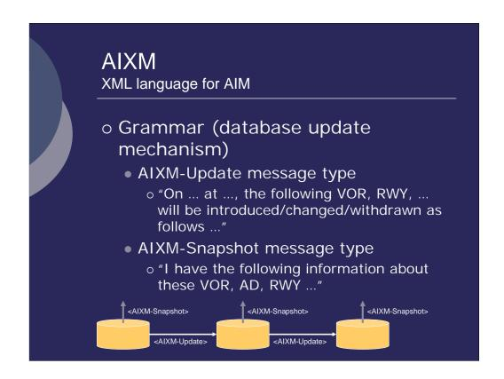
AIXM also includes a grammar. AIXM 4.5 has a limited grammar based on database management and synchronization. The <AIXM-Update> message type allows a system to indicate new, removed or updated features. For example, "on April 1, 2006 the following VOR, RWY, IAP will be added and the following SIA and RSG will be updated."
