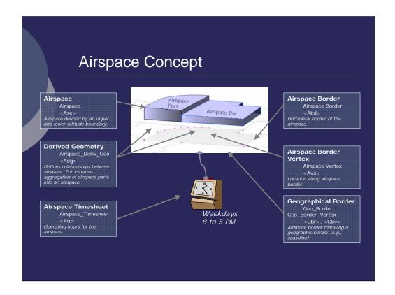
According to the AICM Manual, "Airspace is a generic entity representing variously 'regions' (ICAO and otherwise), 'areas', 'zones', 'sectors' (elementary and/or consolidated)..." Basically the airspace concept can be used to represent any three dimensional geographic space. Examples: FIR, air traffic control sector, an ARTCC boundary, a military operating area or a temporary flight restriction.
