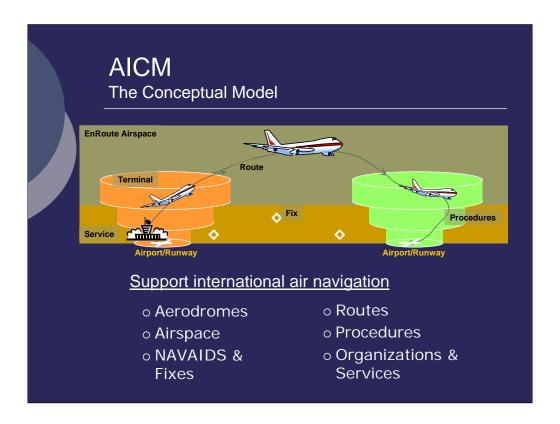
The role of AICM is to enable systems to manage aeronautical information and to enable humans to communicate and understand the information that is managed. AICM describes the features, properties and relationships in a number of conceptual areas as indicated on the diagram.
