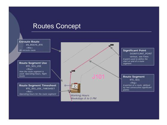
The Routes data concept area is used to define an en-route routes. Within the United States this includes jetways and airways used to traverse the en route airspace structure. Note that approach procedures and departure procedures are modeled separately in the procedures data concept area.
