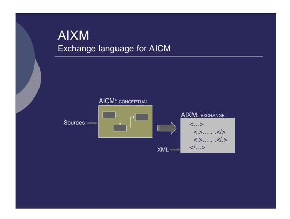
AIXM derives from AICM by mapping the AICM features, properties, relationships and rules into XML.
