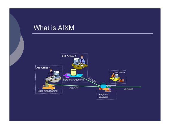
AICM is not enough, we need a standard way to encode the information so a computer can transmit and receive it. AIXM is based on AICM and it is the system to system exchange specification for aeronautical information. AIXM is based on XML.
