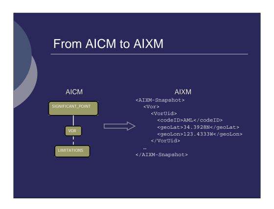
AIXM is the physical implementation of AICM in XML (Extensible Markup Language). The diagram shows how the VOR entity-relationship diagram is converted into AIXM. In AIXM, the VOR is called a feature.
